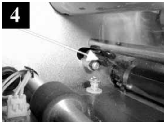
4 Ensure that the film passes between the forks of the optical sensor.
